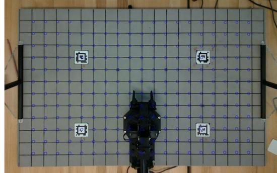
Fig. 4: Grid-points Projection on Warped Image
